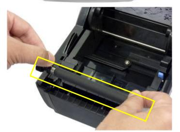
The **Platen Roller is used to** hold the media roll, usually labels.
