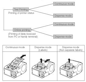
You can select **Dispense mode** for non-separate labels by using the printer setting tool.
