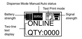
**Battery strength:** Three-segment indicator. When all segments are lit, voltage level is greater than 8.0 V. Two segments indicator a level of between 7.8 V and 7.9 V. One segment indicates a level of between 7.6 V and 7.7 V. When all segments are off (voltage level below 7.5 V, printing is not possible.)
