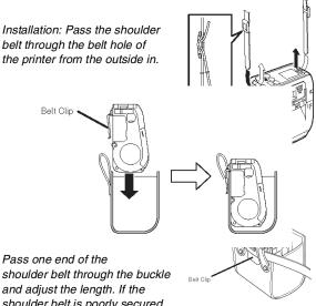
and adjust the length. If the shoulder belt is poorly secured the printer to may fall off.
