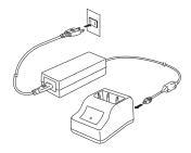
1. Connect the power cord to the charger unit, then plug it into the outlet.
