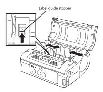
3. Load the paper in the printer. Make sure the roll is oriented correctly.
