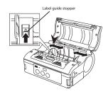
3. Peel the label at the tip of the label paper. This step is unneccessary when you are using linerless labels.
