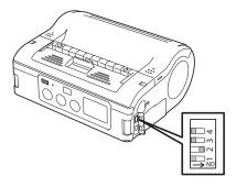
1. Remove the USB/DIP switch cover, and set the DIP switch (DSW) to DSW-1, 2, 3, 4 = (OFF, ON, OFF, OFF).
