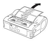
1. Slide the cover release lever in the arrow direction to open the cover. First, slide the dispenser unit to the continuous printing mode position. (See Switching from Dispense mode printing to Continuous printing mode, in this section, Preparing for First-time Operation.)
