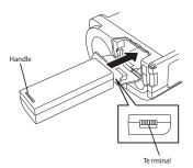
2. While pressing the gray hook, insert the battery pack, then close the battery cover.
