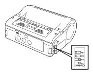
1. Remove the USB/DIP switch cover, and set the DIP switch (DSW) to DSW-1, 2, 3, 4 = (ON, ON, OFF, OFF).
