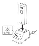
2. Insert the battery pack into the slot, with the terminal pointing downward.
