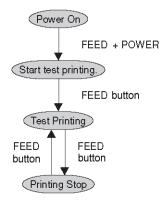
LED indication at the test print mode is as shown below.
