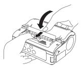
5. Check that the label tip is protruding. Then close the main cover by pressing the middle of the cover. Close the main cover slowly, while pulling the cover release lever.
