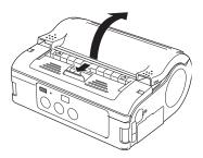
2. While pressing the label guide stopper, slide the label guide to the label size to be used.
