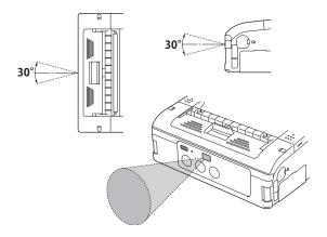
3. Adjust the printer position so that the PC or handheld terminal is within a 30° area vertically and horizontally (cone shape) from the center of the infrared communication sensor
