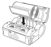
4. Confirm that the label roll can be rotated easily by hand. If rotation is labored, this can cause a feed error. Remove the label roll and adjust the label guide. Note that the label guides do not require adjustment when you are using labels with the same width.
