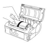
6. Check that the label tip is protruding (10 mm or more). Then close the main cover by pressing the middle of the cover. Close the main cover slowly, while pulling the cover release lever.
