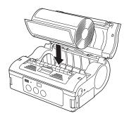
5. Confirm that the label roll can be rotated easily by hand. If rotation is labored, this can cause a feed error. Remove the label roll and adjust the label guide. Note that the label guides do not require adjustment when using labels with the same width.
