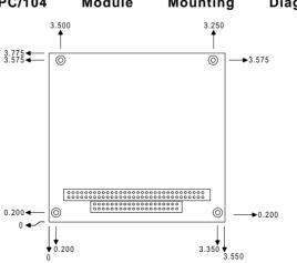
Step5 Secure the PC/104 module onto the CPU card using the four mounting spacers and srews.
