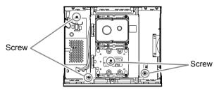
If the HDD block was removed in step 4, reattach.
