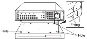
(2) Use the remaining screw (accessory) to secure the fitting on to the right side of the DVR.
