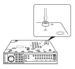
4 Remove the four screws from the sides of the DVR, and remove the cover.
