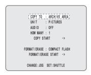
3 Turn the jog dial to select "FORMAT/ ERASE", and then turn the shuttle dial clockwise.
