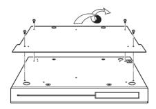
2 Use two screws (accessory) to attach the fitting (accessory) to the external disc unit.
