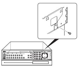
6 Use the four screws removed in step 1, to secure the DVR from the inside to the external disc unit.
