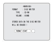
6 Turn the jog dial to select "FORMAT START", and then turn the shuttle dial clockwise.
