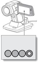
If you swivel the monitor unit to its farthest position, the image on the monitor will be inverted.
