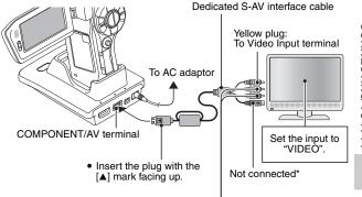
White plug: To Audio Input (L) terminal Red plug: To Audio Input (R) terminal
