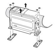
• Once more, use the hexagonal nuts to attach the changer on top of the carpet.
