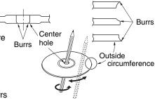
Remove all plastic particles of burr from surfaces of disc before loading in magazine.
