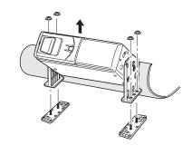
• Once more, use the hexagonal nuts to attach the changer on top of the carpet.
