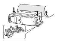
Remove the hexagonal nuts and take off the changer.
