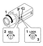
**F** Flange-back adjustment screw (FLANGE BACK ADJ.)
