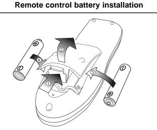
Install two "AA" 1.5 volt batteries so that the "+" and "-" marks on the batteries match the "+" and "-" marks inside the unit into the remote control handset.
