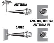
The tuner in this HDTV can receive: • Digital and Analog off air signals from an antenna
