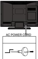
To the AC Outlet (100-240V AC) Pulls the AC power cord out from the LCD TV. The AC outlet must be near this equipment and must be easily accessible.
