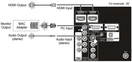
NOTE : You can connect the DVI source to HDMI input terminal by using the DVI to HDM I converter, and you just can watch image, but without sound.
