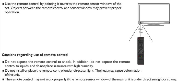
The remote control may not work properly if the remote sensor window of the main unit is under direct sunlight or strong lighting. In such a case, change the angle of the lighting or the TV set, or operate the remote control closer to the remote sensor window.
