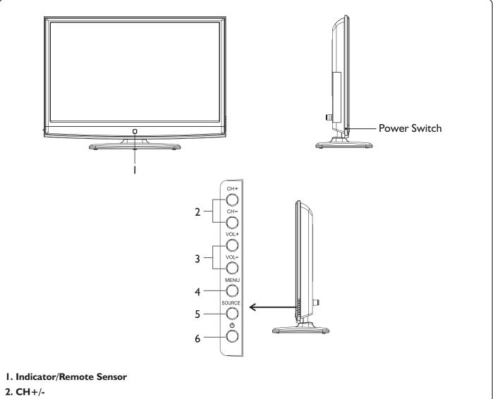
Press these two buttons to directly change the TV channel;
