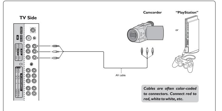
Connect the Audio/Video cables between the Audio (L/R)/Video jacks on the unit and camcorder.
