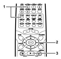
1. Press [PLAY MODE] while holding [SHIFT] down during playback or stop mode.
