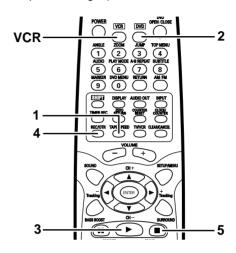
Press [TAPE SPEED] to select the desired tape speed SP or SLP.
