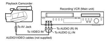
For duplicating a previously recorded tape from a camcorder, follow the camcorder manufacturer's instructions. A typical camcorder dubbing hookup is shown above.
