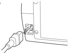
**2** Remove the connector cover and screw covers from the projector and insert plug on this product to the option connector.
