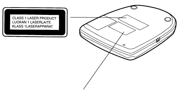
The rating label is located on the bottom of the unit.
