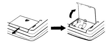
2. Insert the NBP-50A rechargeable nickel-cadmium battery (not supplied) into the battery compartment. Be sure to observe the proper polarity (the "+" and "-" signs, as indicated inside the battery compartment).
