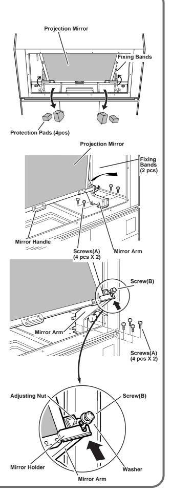
When the figure of the projection image does not match the Projection Screen, adjust the Projection Mirror. If the figure fits the Projection Screen precisely, skip the steps 2, 3 and 4 and replace the Back Cover.
