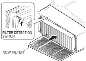
4 Check that the filter is not tilted or warped and then close the filter cover. This will lock it into place.
