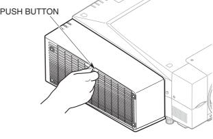
2 Open the filter cover and take out the used filter.
