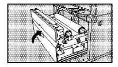
Turn the knob until the paper edge extrudes from the cover by about 150mm. 5.9" (cover closed).
