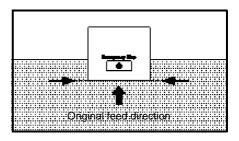
Press the Partial Copy key when the trailing edge of the area to be copied comes to the position where it is covered with the original table cover.
