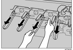
**8** Remove the securing pin, as shown, from the transfer unit. Pinch it, and then pull it out.
