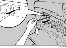
9 Turn the green lever of the transfer unit counterclockwise to unlock the unit.
