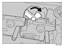
**12** Close the inner cover. Lock the inner cover by pressing in (①) and then turning the two green levers clockwise (②).
