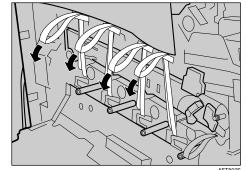
Remove the four pieces of tape from the photo conductor unit.
