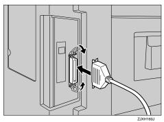
Plug the other end of the parallel cable into the computer's parallel port. If there are the wire clips, squeeze them on each side of the connector together.
