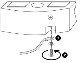
Note: Use a grounding strip or a conductor with a cross-section of 1 to 1.5 mm<sup>2</sup> (AWG18, AWG16) and a length of  $\leq$  3 m (9.84 ft) long. The maximum recommended length for the grounding strip is 3 m (9.84 ft).
