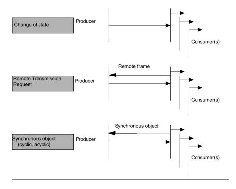
**Synchronous** For certain applications, synchronization between scanning of the inputs and activation of the outputs may be necessary.
