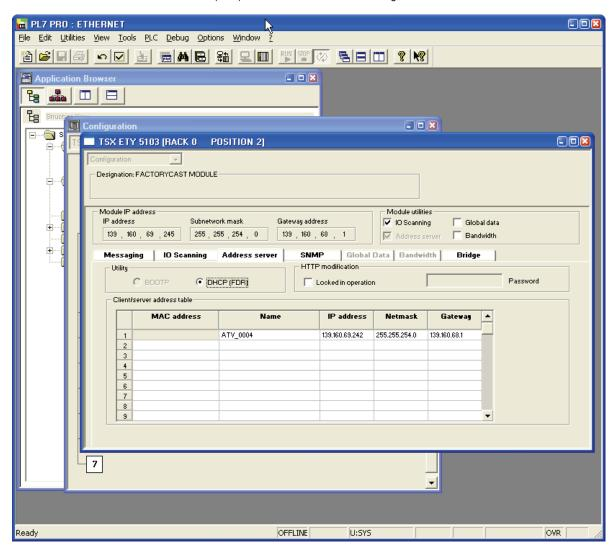
This window is used to configure the DHCP server.
