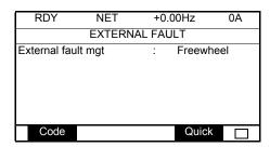
The values of parameters: [COM. fault mgt] (*LL*) that will trigger a stop response from the drive [Com. network] (*LR*) and [External fault mgt] (*EPL*) that will trigger a stop response from the drive [External fault com.] (*EPF2*) are: [Freewheel] (*YE*5): Freewheel stop (factory setting). [Ramp stop] (*RP*): Stop on ramp. [Fast stop] (*FSE*): Fast stop. [DC injection] (*LL*): DC injection stop.
