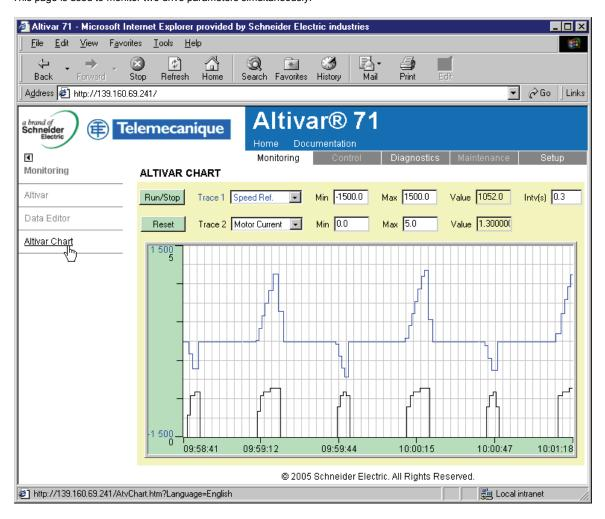
Two parameters can be selected and displayed simultaneously. To do this, select them in the Trace1 and Trace2 list.
