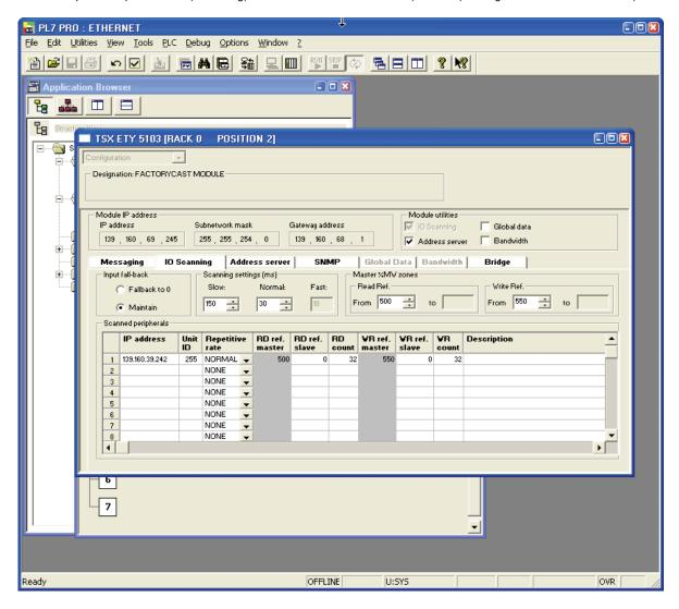
The addresses for the PLC %MW words correspond to the configuration in the previous example.
