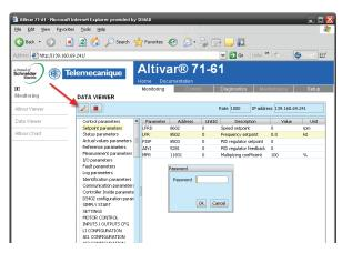
It is only possible to modify the parameter values after entering the "Write password" (see "HTTP password" and "Data write password pages" section on page <u>55</u>). Click on the "Password" button to enter this password. An entry field then appears in the parameter table, and also a "Cancel" button, for canceling the password entry. After entering the password, press the Enter key so that it is taken into account by the web browser.
