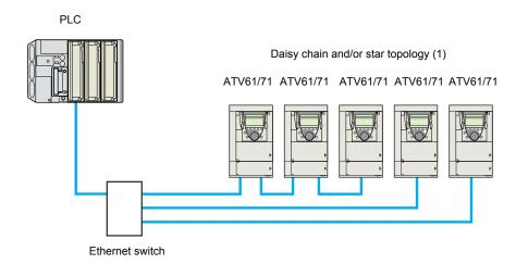
(1) When the topology is a daisy chain, if one drive is turned off, the other drive(s) stop in response to a communication network fault (CNF).
