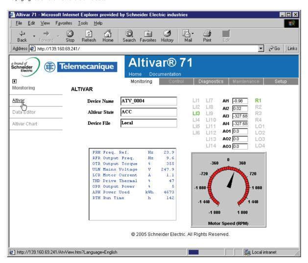
The state indicated in the "Altivar State" field corresponds to the display on the drive integrated display terminal. A delay may sometimes be noticed between the displays on the web server and the display terminal, depending on the performance of the computer used to display the pages using a web browser and the communication system performance.
