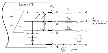
\*3 x 230 V +10% max. with a BPH055 Servo motor
