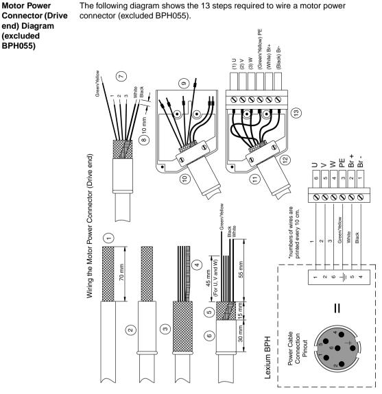
The following diagram shows the 13 steps required to wire a motor power
