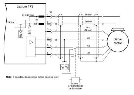
BRAKING RESISTORS - To determine the values of the braking resistors, use these formulas:
