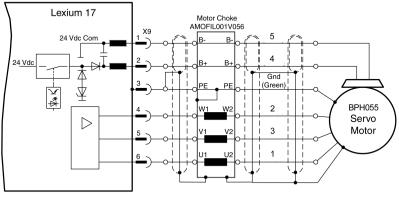
Note: The choke must be installed at a distance of one meter or less from the drive
