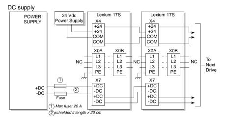
Notes: -Inrush current must be limited to 20 A between power supply and drives. - Drives have to be configured (see Unilink commands) to suppress faults.
