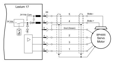
Connection between servo motor and drive when interface cable length exceeds 25 m.
