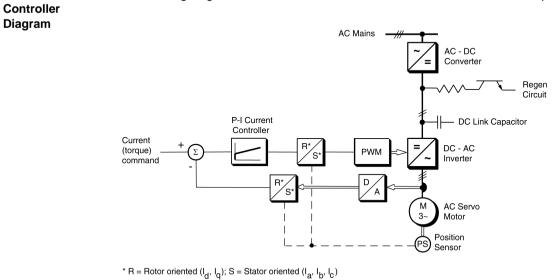
The following diagram shows an overview of the 17S current controller servo loop.
