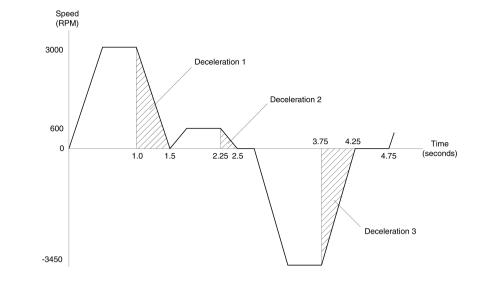
**Example Step 2** Identify each deceleration of the plot where the drive is decelerating the load.
