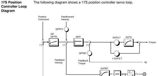
The following diagram shows a 17S position controller servo loop.
