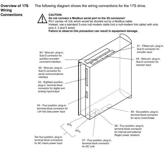
**Note**: The connectors described above appear in many wiring diagrams throughout the remainder of this document and are identified in those diagrams by their alphanumeric designations only (for example, X4); the term *connector* is excluded.
