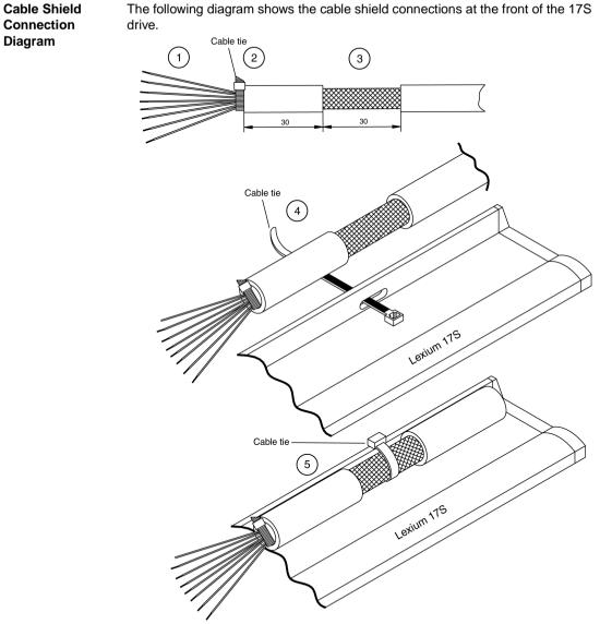
The following diagram shows the cable shield connections at the front of the 17S
