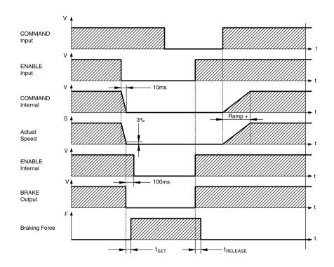
During the fixed ENABLE delay time of 100 ms, the speed setpoint of the drive is internally driven down a 10 ms ramp to 0V. The 3 % region of actual speed is scaled to  $V_{LIM}$ .
