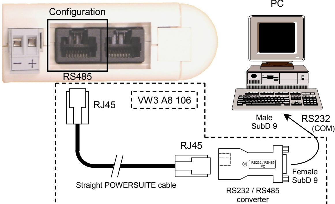
Once the gateway has been connected to a PC with the PowerSuite cable and the RS232/RS485 converter, you can change its configuration using "ABC-LUF9 Configurator", more generally referred to as "AbcConf". This configurator also allows you to carry out a few diagnostics on the gateway.
