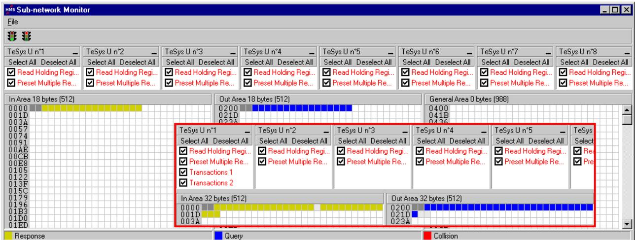
You will note that the "TeSys U n°1" section now only has the two Modbus commands common to the eight TeSys U motor starters, and that the memory locations which corresponded to the two personalised commands are now free.
