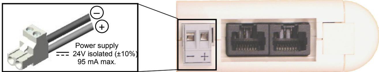
We do not recommend powering the gateway using the 24V power voltage  $\equiv$  on the DeviceNet network. It is better to use a separate power supply, because the gateway needs to be powered using a stabilised voltage, which is not necessarily the case with the power voltage on the DeviceNet network.
