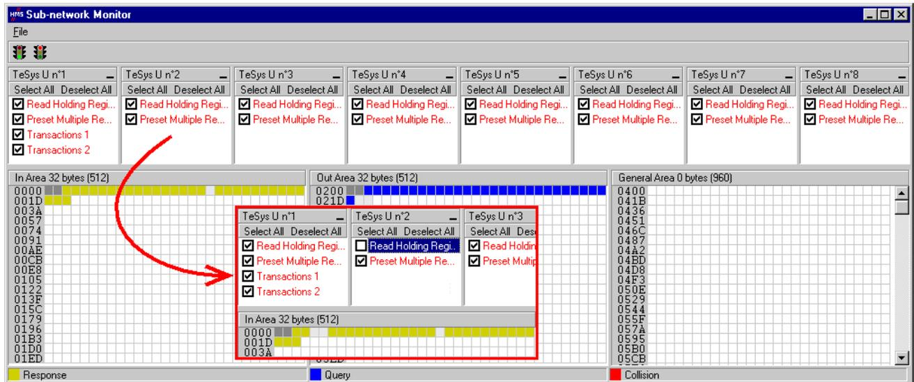
To see which memory locations are occupied by data from the command you are interested in, all you have to do is uncheck the box corresponding to the "Read Holding Registers" command from the "TeSys U n'2" node, as shown above. We can see that the Modbus data received in response to this command occupy 2 bytes located from address 16#0004.
