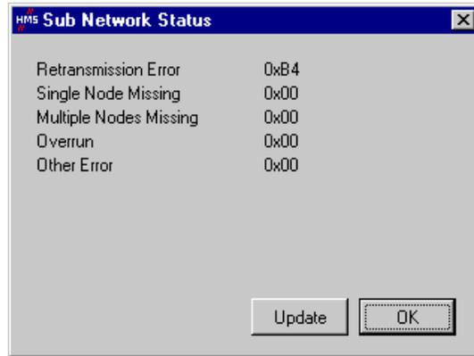
When you run this command in "off-line" mode, all of the values displayed are replaced by the word "Unknown" to show that they cannot be read on the gateway. The "Update" button then becomes inaccessible.
