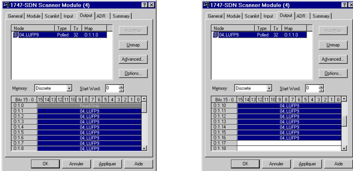
The correspondence between the contents of the gateway’s output memory (see chapter 8.2.2 Output Data Memory Area, page 85) and PLC outputs “O:1.1” to “O:1.16” is given in the following table:
