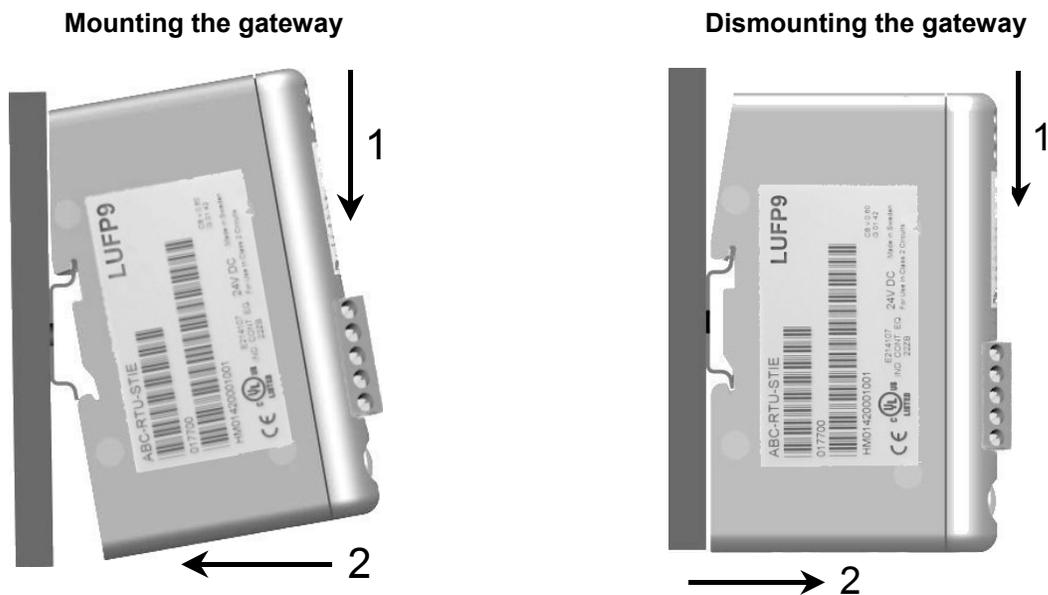
Start by fitting the rear base of the gateway to the upper part of the rail, pushing downwards (1) to compress the gateway's spring. Then push the gateway against the DIN rail (2) until the base of the gateway box fits onto the rail.
