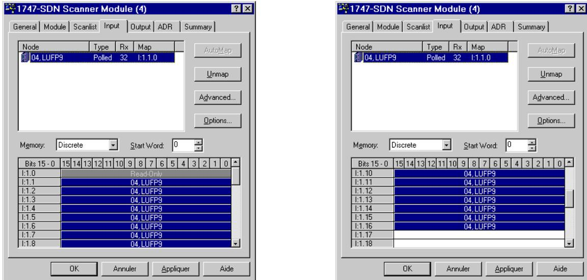
The correspondence between the contents of the gateway’s input memory (see chapter 8.2.1 Input Data Memory Area, page 84) and PLC inputs “I:1.1” to “I:1.16” is given in the following table:
