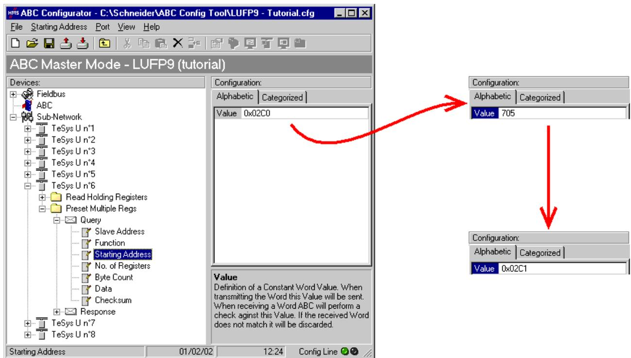
This operation in no way changes the content of the gateway’s memory, because we do not need to change the values of the “Data length” and “Data location” fields of the “Data” element of the “Query”. So no additional operations will be necessary, either in AbcConf, or in RsNetWorx.
