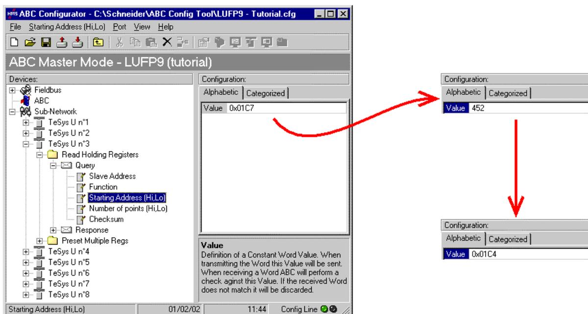
This operation in no way changes the content of the gateway’s memory, because we do not need to change the values of the “Data length” and “Data location” fields of the “Data” element of the “Response” to the aforementioned command. So no additional operations will be necessary, either in AbcConf, or in RsNetWorx.
