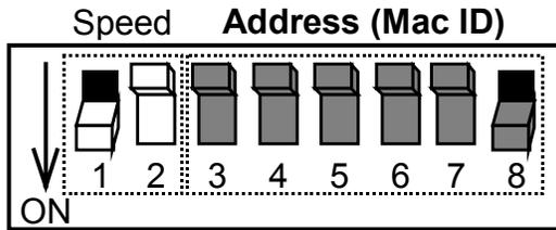
The gateway's DeviceNet address depends on the position of selector switches 3 to 8. It corresponds to the binary number given by the ON (1) or OFF (0) position of these 6 selector switches.
