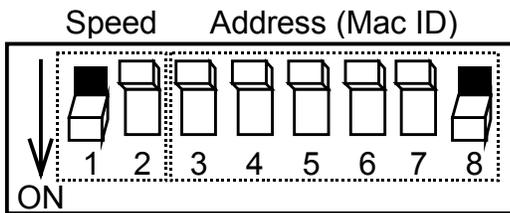
A selector switch is in the 0 state when it is in the OFF position and in the 1 state when it is in the ON position.
