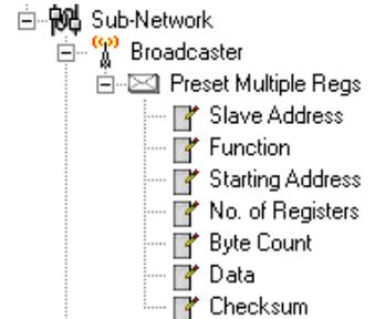
The addition and configuration of a Modbus command in the list of broadcaster node commands is done in the same way as for other nodes, but with the following differences:
