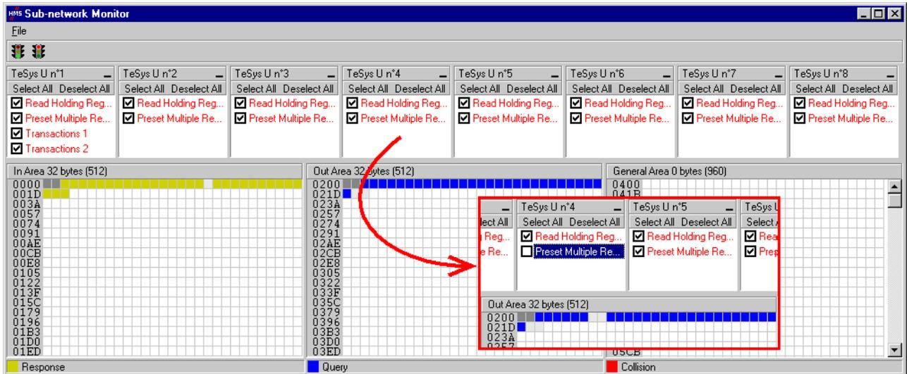
To see which memory locations are occupied by data from the command you are interested in, all you have to do is uncheck the box corresponding to the "Preset Multiple Registers" command from the "TeSys U n°4" node, as shown above. We can see that the Modbus data transmitted with the query corresponding to this command occupy 2 bytes located from address 16#0208.
