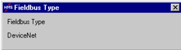
In “on-line” mode (see chapter 6.12.2 “ABC” Element, page 76), the window shown opposite will be displayed. In “off-line” mode the word “Unknown” will replace “DeviceNet” to show that the type of upstream network cannot be identified.
