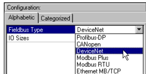
If your PC is connected to the gateway using the PowerSuite cable and you are using AbcConf in "on-line" mode when AbcConf starts up, the type of upstream network will be automatically detected.
