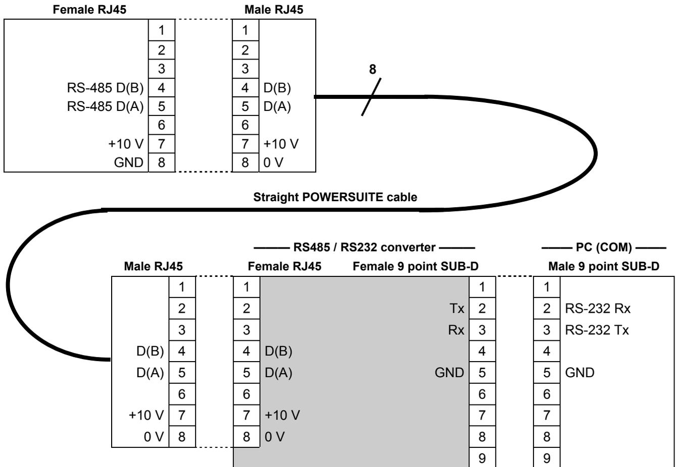
**N.B.** The inversion of the Rx and Tx signals between the gateway and the PC is shown on the 9-point SUB-D connectors, because beyond this junction, the RS-232 signals are replaced by the D(A) and D(B) polarisations of the RS-485 signals.
