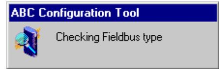
Once this test has finished, a window called “Download” opens and a progress bar shows the state of progress for the transfer of the configuration to the gateway. You must never interrupt this operation, otherwise you will have to start it again from the beginning.
