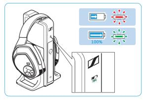
When not in use, place the headphones on the headphones holder to ensure that batteries are fully charged when needed. The transmitter utilizes an intelligent battery charging technology that prevents overcharging.
