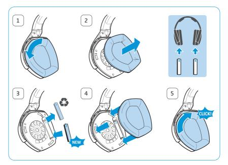
You can also power the headphones using standard batteries (AAA size, 1.5 V). Note however, that standard batteries are not rechargeable, and if you are using non-rechargeable batteries, you must not place the headphones on the headphones holder.
