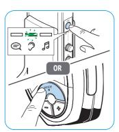
5 Use the rotary switch to select a hearing profile A-G and test which of the hearing profiles gives you the best sound quality and helps you to hear best.
