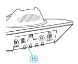
➤ Set the ST/MO switch (16) of the transmitter to MO (mono).
