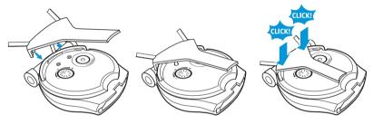
► Connect the induction loop to the socket ⑦ of the receiver.
