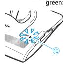
If the operating mode was changed successfully, the charging indicator for the spare rechargeable battery (10) goes off and the indicator (14) lights up again.
