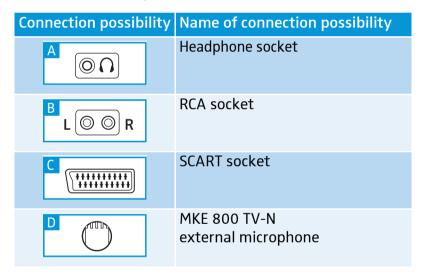
Connect the transmitter as described in the corresponding chapter A, B, C or D.
