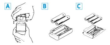
Connect the battery pack to the transmitter. The battery pack locks into place with an audible click.
