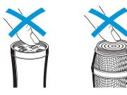
When unscrewing the microphone head 1 during operation, the muting function is automatically activated. "MUTE" appears on the display panel.
