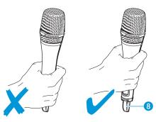
Only hold the radio microphone by its body.
