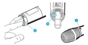
To switch the radio microphone on (online operation):
