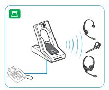
▶ Place the base station at a minimum distance of 15 cm from the fixed line phone.
