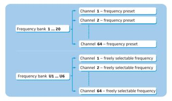
Each of the channels in the frequency banks "1" to "20" has been factorypreset to a fixed receiving frequency (frequency preset). The factorypreset frequencies within one frequency bank are intermodulation-free. These frequencies cannot be changed.
