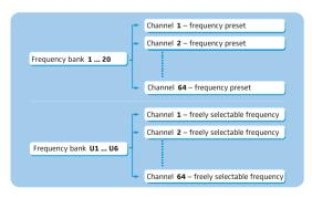
Each of the channels in the frequency banks "1" to "20" has been factory-preset to a fixed frequency (frequency preset). The factory-preset frequencies within one frequency bank are intermodulation-free. These frequencies cannot be changed.
