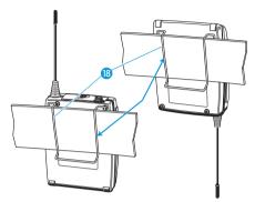
The belt clip is detachable so that you can also attach the transmitter with the antenna pointing downwards. To do so, withdraw the belt clip 18 from its fixing points and attach it the other way round.
