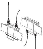
The transmitter is attached to dothing (e.g. belt, waistband) with the supplied belt clip.
