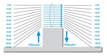
This transmitter is equipped with HiDyn *plus* the Sennheiser noise reduction system that reduces RF interference. It increases the signal-to-noise radio in wireless audio transmission to more than 114 dB.
