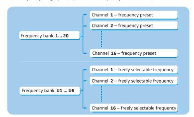
Each frequency range (A–E, G) offers 26 frequency banks with up to 16 channels each:
