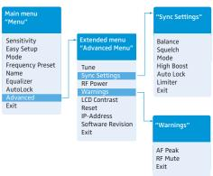
When the standard display is shown on the display panel, you can get into the main menu by pressing the jog dial. The extended menu "Advanced Menu" and the other menus can be accessed via the corresponding menu items.
