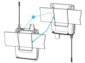
The belt clip is detachable so that you can also attach the diversity receiver with the antenna pointing downwards. To do so, withdraw the belt clip from its fixing points and attach it the other way round. The belt clip is secured so that it cannot slide out of its fixing points accidentally.
