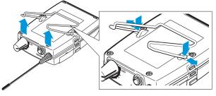
Press down the belt clip at one fixing point and pull it out of the receiver housing.
