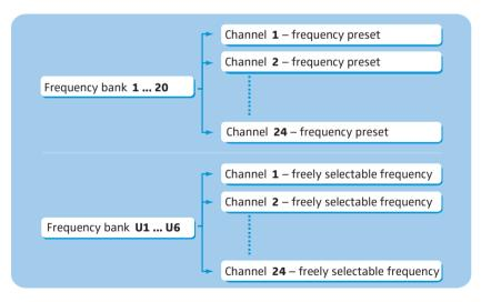
Each of the channels in the frequency banks "1" to "20" has been factorypreset to a fixed frequency (frequency preset).
