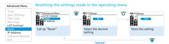
When resetting the settings made in the operating menu, only the selected settings for the pilot tone and for the frequency banks "U1" to "U6" remain unchanged. For an overview of the factory-preset default settings, refer to the supplied frequency information sheet.
