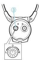
The balance control allows for right/left balance adjustment. Adjust the balance so that you can hear equally well with both ears.
