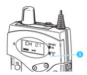
The green LED (RF) 5 at the front of the receiver lights up when an RF signal is being received.
