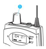
Switch the receiver off to exit the setup menu. To do so, turn the volume control 1 counterclockwise until it clicks
