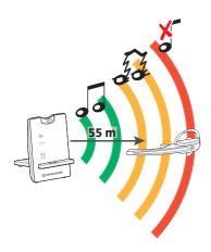
In normal office buildings, the range between headset and base station is up to 55 m. If, during a call, the audio quality deteriorates or the link breaks down completely, you hear a descending sequence of beeps in the headset. The Link LED  $\bigcirc$  on the base station lights up red.
