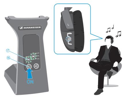
If the transmitter doesn't receive an audio signal for more than 3 minutes, it switches, depending on the setting, to either standby mode or loop through mode. If the transmitter receives an audio signal within the next 10 minutes, it automatically switches on again.
