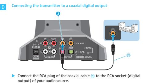
Connect the RCA plug of the coaxial cable 23 to the COAXIAL IN input 3.
