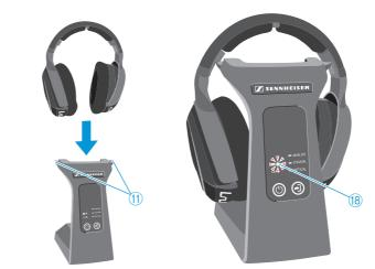
Place the headphones on the charging contacts (1) of the transmitter. The rechargeable batteries are being charged. The Battery LED (18) lights up red.
