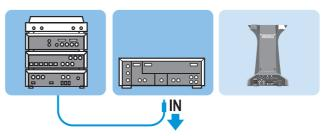
Connect this plug to a suitable input ("IN") on the transmitter (see page 7).
