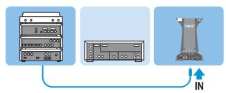
Connect an additional identical audio cable to the output ("OUT") on the transmitter and to the input ("IN") on the amplifier.
