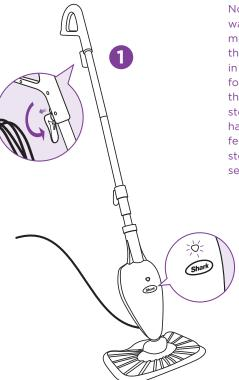
Now comes the part you've been waiting for – it's time to use your steam mop. When you use your steam mop for the first time or haven't used the unit in awhile, it may take a minute or two for the water to make its way through the pump and into the heater to create steam. Get it started by pumping the handle a few times. If you've waited a few minutes and you still don't see any steam, reference the troubleshooting section on page 9.
