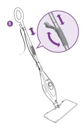
5 For your comfort, you can adjust the height of the mop. Just lift the latch on the tube 90 degrees to the open position. Holding the handle, extend the tube to the height that's right for you and then close latch to locked position. **QUICK TIP:** For easier pushing and pulling, extend the handle length.
