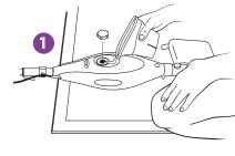
1 Turn the water tank cap counter clockwise and remove from the tank.
