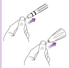
Cleaning tip: To prevent clogging, it is recommended that you periodically clean the Direct Steam Nozzle and the extension hose stem with the cleaning tool provided or a paper clip.
