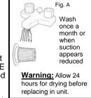
then rinsed under the faucet and allowed to air dry for 24 hours before replacing into the vacuum. (Fig. A) This should be done once a month or when suction appears to be reduced.
