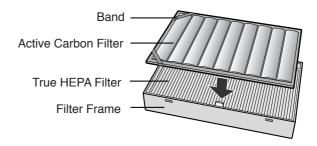
3 Place the Pre-filter through the bands (2 places) located in the corners of the Active Carbon Filter.
