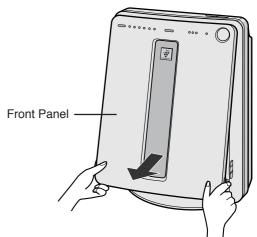
2 Pull out the Filter Frame and remove the Pre-Filter, Active Carbon Filter and True HEPA Filter.
