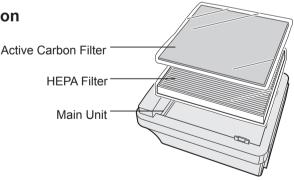
Remove the Active Carbon Filter and HEPA Filter from the plastic bags.
