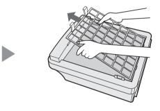
Remove the Active Carbon Filter and HEPA Filter.
