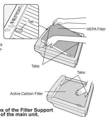
3 Insert the bottom side tabs of the Filter Support into the associated holes of the main unit. Next push the upside tabs into the main unit.
