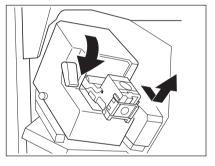
Remove the empty staple case upward from the staple cartridge.
