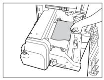
Lift the grip, then turn the knob in the direction of the arrow to remove any misfed paper.
