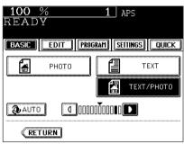
When the DENSITY LEVEL key is shown on the lower left of the screen, you can adjust the density manually on the basic screen.
