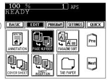
Select the orientation (Short edge or Long edge) and position of the page number to be printed. Then, press the SET key.
