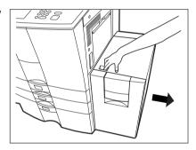
Remove any misfed paper by turning the blue knob in the direction of the arrow.
