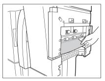
6 Open the tray of the inserter to remove any misfed paper.
