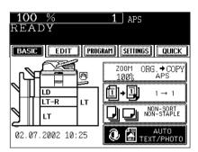
Choose the desired image type mode by pressing one of the PHOTO, TEXT, and TEXT/PHOTO keys.
