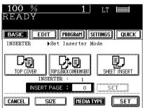
Press the key of the paper size placed in the inserter, then press the RETURN key.
