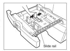
Push the arrow part (right side) of the size selection lever to unlock it.
