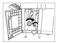
6 Remove any paper misfed on the exit side of the saddle stitch unit.
