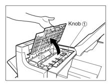
**2** Lift knob ① (See the upper right figure), then remove any misfed paper.
