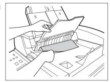
T Lifting the handle in the direction of the arrow, pull it toward you.
