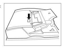
Rotate the blue knob to remove any misfed originals.
