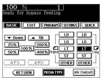
After selecting the media type key corresponding to the type of the paper that has been set, press the SET key.
