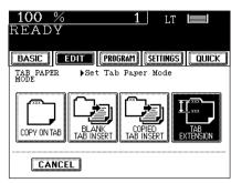
Press the CASSETTE key (or the BYPASS FEED key), then adjust the tab extension (tab width) and the shift width then press the SET key.
