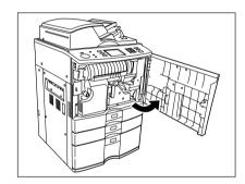
Rotate the left end of the holder, then pull out the empty toner cartridge with both hands as shown on the right.
