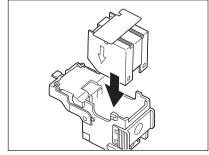
Pull out the seal holding the staples straight upward.
