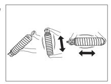
Holding the new toner cartridge as shown on the right, pull out the seal in the direction of the arrow.
