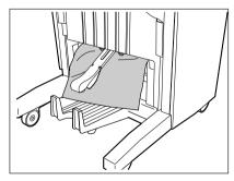
Open the exit cover of the saddle stitch unit and remove any misfed paper.
